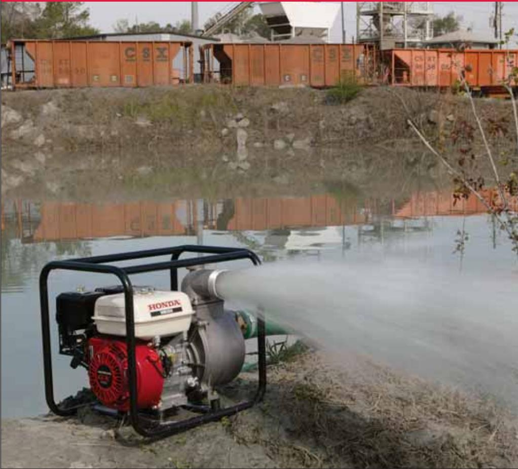
Honda's WB series pumps offer the best features at a value price. Featuring Honda's commercial-grade engine and rugged full frame protection with anti-vibration mounts, these pumps feature a fixed-mounted cast iron volute and impeller with a silicon carbide seal. This is the ultimate combination of features to provide unsurpassed performance and durability in the toughest conditions.
